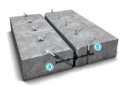
**Borepacker arrangement:** Drilled holes with inserted packers crossing construction joints through the joint strip flange. Techniques (A)+(B)
