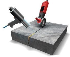
**Gravitational filling:** Gravitational filling is performed under pressureless conditions (and without packers). Wide cracks can be filled without preparation, whereas narrow cracks will need to be ground out first.
