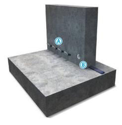
Borepacker and hose injection: Packers arranged at intervals corresponding to half the component thickness at an angle of 30–45° to access the joint. (A)
