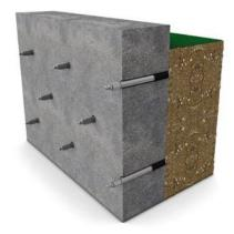
**Borepacker use:** Packer arrangement for concrete interfaces
