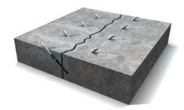
Borepacker drill hole packers: These are inserted in the drilled holes at a distance corresponding to half the crack depth in a staggered formation on both sides of the crack (usually without surface sealant).
