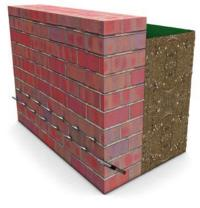
Borepacker use: Packer arrangement for masonry
